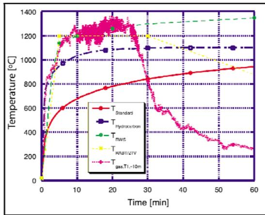
FIG. 2: STANDARD CURVES <-> REAL FIRE CURVE
