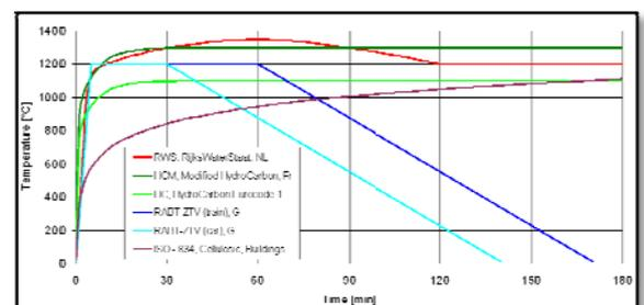
FIG. 1: COMMON USED FIRE-CHARACTERISTIC CURVES
