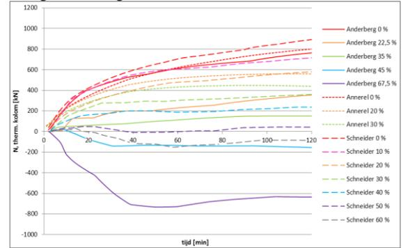
Figure 4:  $N_{therm, column}$  during heating following the ISO 834 curve
