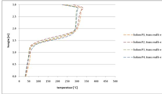
Figure 2: Temperature development in function of height for 4 different columns.
