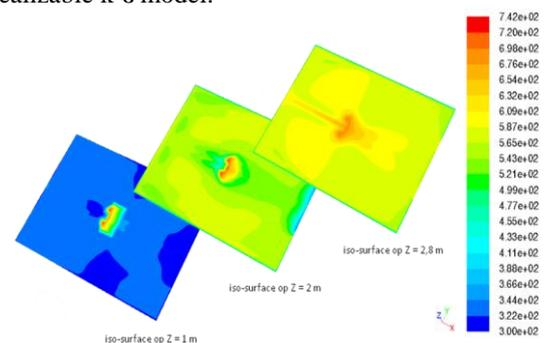
**Figure 1:** Temperature development at a height of 1m, 2m and 2.8m for a burning car in the middle with a realizable k- $\epsilon$  model
