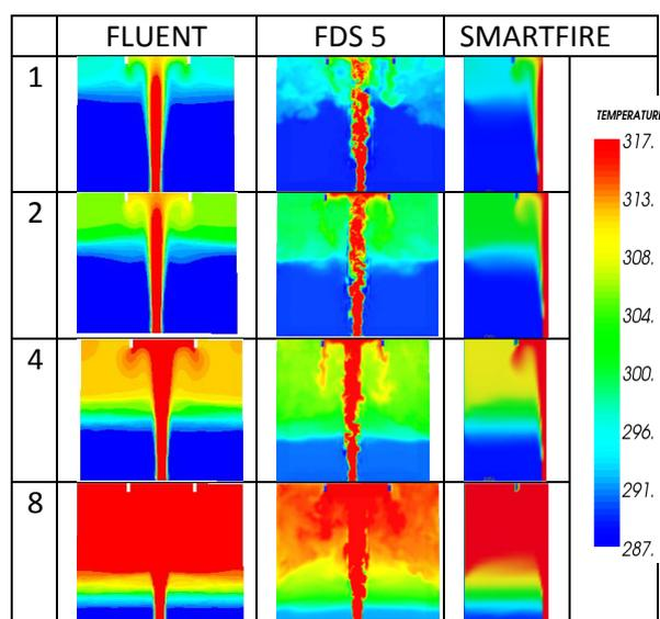
Table 1: Temperature in the middle of the atrium (cross section) after 1, 2, 4 and 8 minutes.
