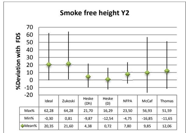
Figure 3 : % comparison of the results obtained with manual formula for smoke free height and the results from FDS.
