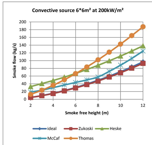
Figure 1 : Comparison of different manual formula for plume entrainment. The heat source is 7.2MW
