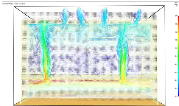
Figure 2 :Vector field showing the entrainment of air in the second compartment (above the compartment with the fire).
