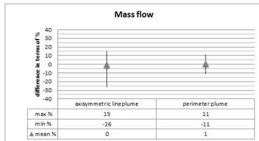
Figure 5 : Difference in terms of percentage for the mass flow (axisymmetric line plume – perimeter plume)
