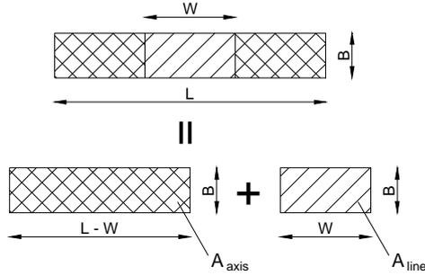
Figure 2 : Ratio area axisymmetric plume and line plume at a height lower than the transition height (i.e.  $0 < z < 3 * (L-B)$ )
