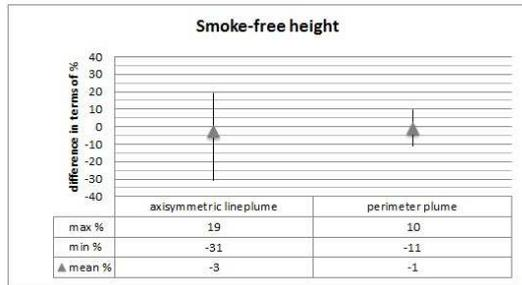
Figure 4 : Difference in terms of percentage for the smoke-free height (axisymmetric line plume – perimeter plume)
