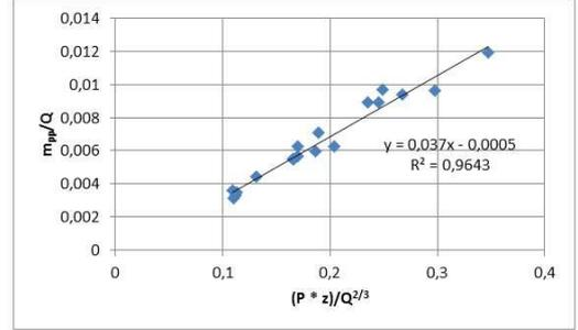
Figure 3 : Determination of the constants A and B on the basis of the obtained results from the FDS simulations
