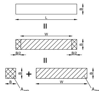
Figure 1 : Ratio area axisymmetric plume and line plume at the opening in the floor (i.e.  $z=0$ )
